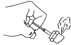
**PILOT VALVE:** When the toggle is in the upright position, all air from the air compressor is vented through the discharge muffler. This gives an easy start feature. For normal operation, the toggle is in the 90° position.
