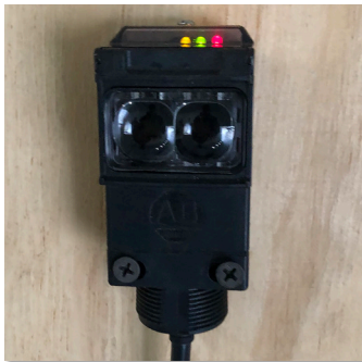
Photo-eye with 10-foot maximum range
